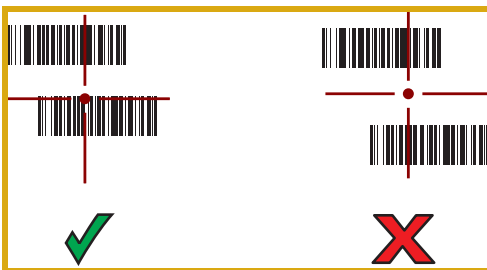
Figure 91 RS6000 Pick List Mode with Multiple Barcodes in Aiming Pattern
