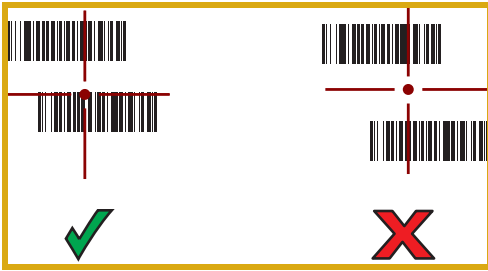
Figure 94 RS507/RS507X Pick List Mode with Multiple Barcodes in Aiming Pattern
