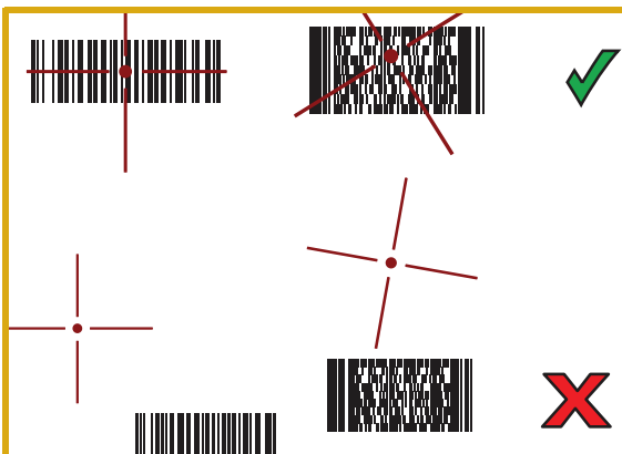
Figure 93 RS507/RS507X Aiming Pattern
