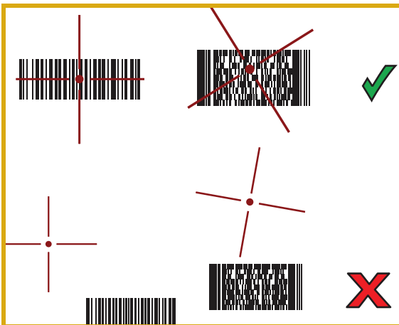
Figure 91 RS6000 Pick List Mode with Multiple Barcodes in Aiming Pattern
